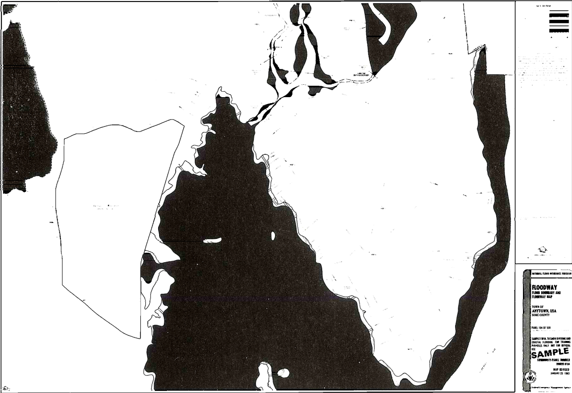
FIGURE 2-4. The Flood Insurance Rate Map (FIRM) and Flood Boundary and Floodway Map (FBFM) pinpoint flood boundaries, flood zones and base flood elevations for a particular community.
